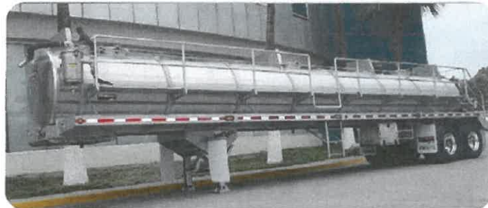
EQUIPMENT: 150 BARREL (6,300 GAL) VACUUM TANK - MADE OF ALUMINUM NEW TRAILER: GALLEGOS® BRAND, CYLINDRIC TYPE VACUUM TANK 150 BBL (6,500 GAL) CAPACITY, 42' LONG x 10.33' HIGH x 8.53' WIDE. YEAR MODEL 2022 WITH THE FOLLOWING SPECIFICATIONS:
